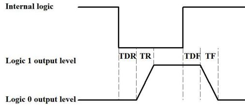
Figure 43 Output logic levels
