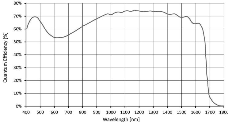
Figure 5 IM991 absolute quantum efficiency
