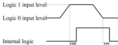
Figure 46 Input logic levels
