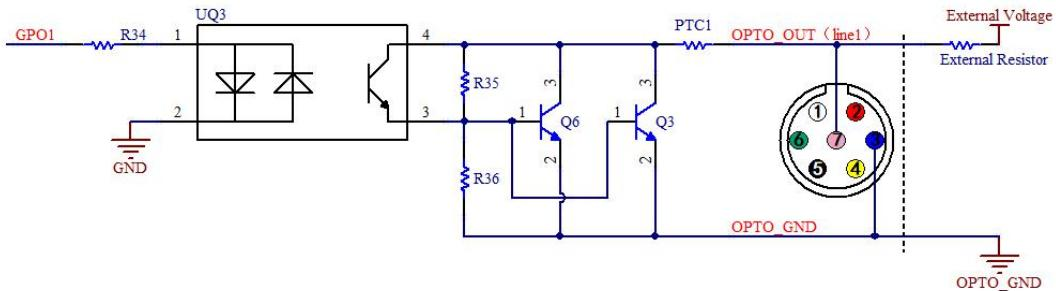
Figure 42 Optocoupler output circuit
