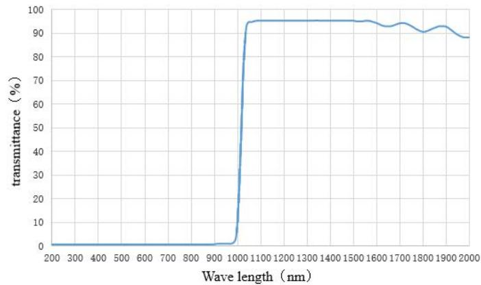
Figure 14 Long wave pass filter LP1000H transmittance curve
