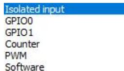
Figure 51 Possible Trigger Sources
