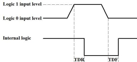
Figure 41 Input logic levels
