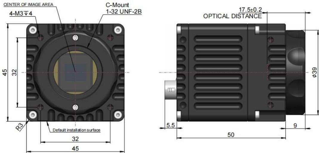
Figure 25 USB port Small size camera dimensions
