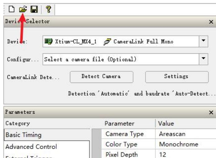
Figure 68 Load the CameraLink receive format configuration information
