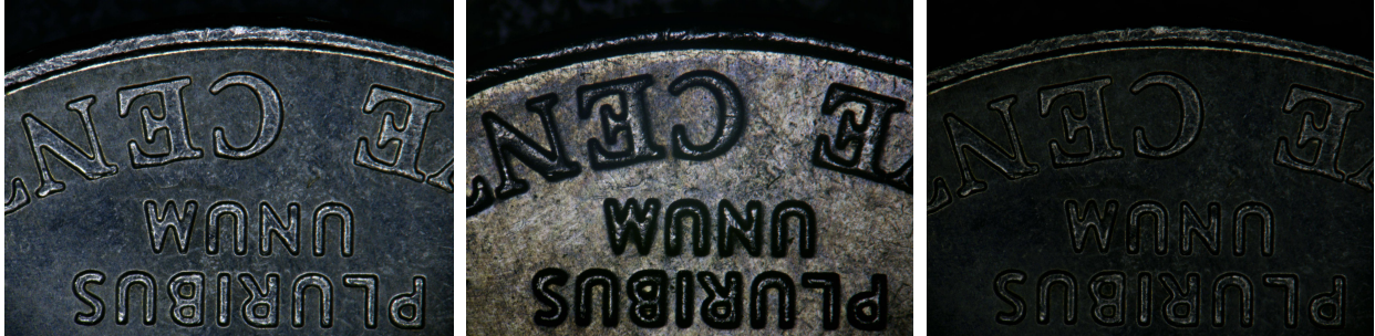
Figure 11 From left to right, there are three pictures of coins taken under left) LED Direct Ring Light illumination; middle) LED Direct Ring Polarization Light illumination; right) Coaxial Light illumination
