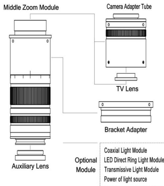
Figure 2 The five basic modules of TZM0440 series MZO.
