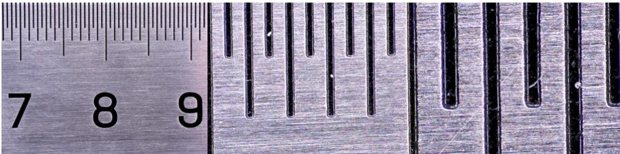
Figure 16 Pictures of steel ruler taken with TZM0440-W3100-TV3050 under LED Direct Ring Light illumination
