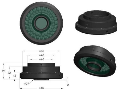
Figure 8 TZM0756DRPL-65, the maximum diameter of the LED reaches 65mm, and the small hole with a center diameter of 40mm can be directly sleeved on the front end of the corresponding MZO. By rotating the polarizing plate, uniform illumination of linear polarized light in different directions can be realized
