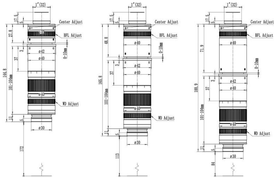
Figure 13 Dimension of TZM0440 series MZO with different Auxiliary Lens and TV Lens
