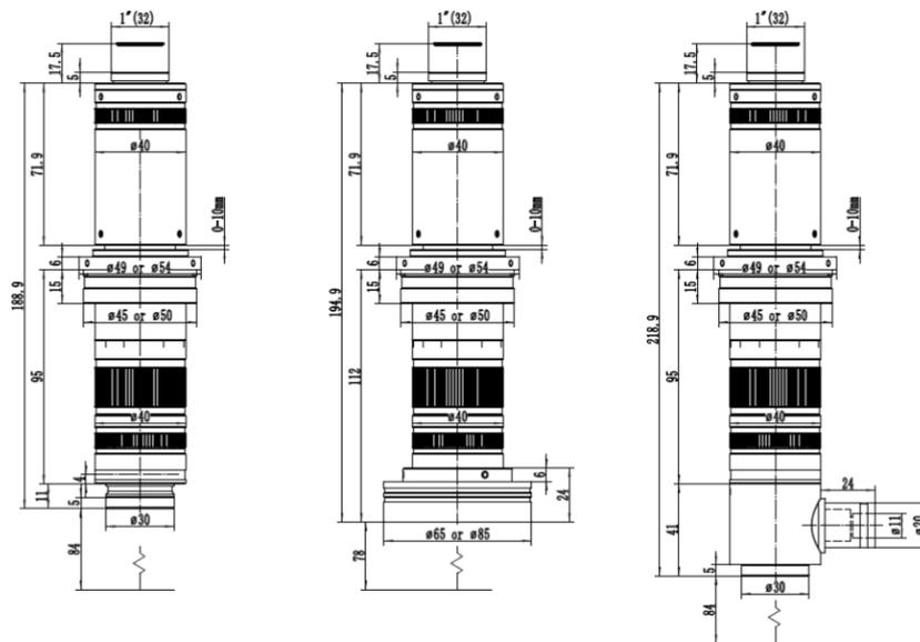
Figure 14 Dimensions of TZM0440-W3100-TV3100-A50 with different light module
