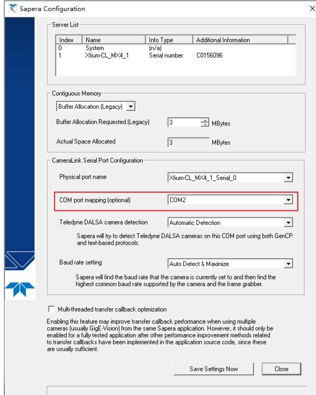
Figure 63 Serial port configuration dialog box
