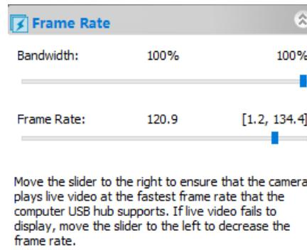
Figure 8 Bandwidth and precise frame rate settings
