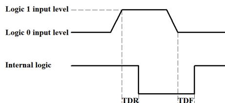
Figure 40 Input logic levels
