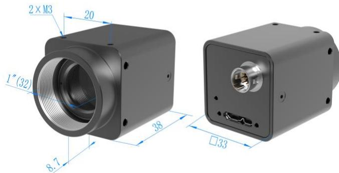
Figure 18 USB interface uncooled camera dimensions
