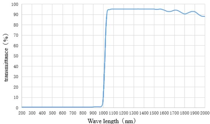
Figure 14 Long wave pass filter LP1000H transmittance curve
