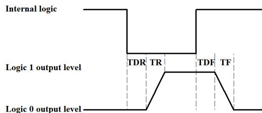
Figure 46 Output logic levels
