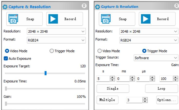
Figure 49 Video Mode and Trigger Mode on the Capture & Resolution group in ToupView
