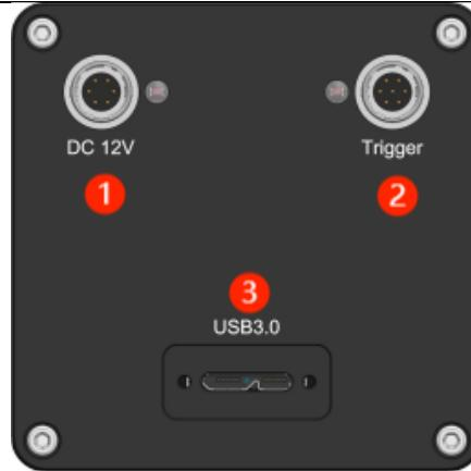
Figure 31 USB interface Cooled Camera
