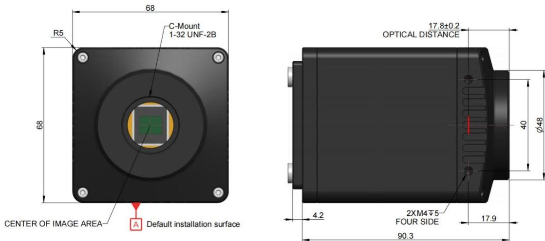
Figure 23 The Front and side view dimensions of the CameraLink interface camera
