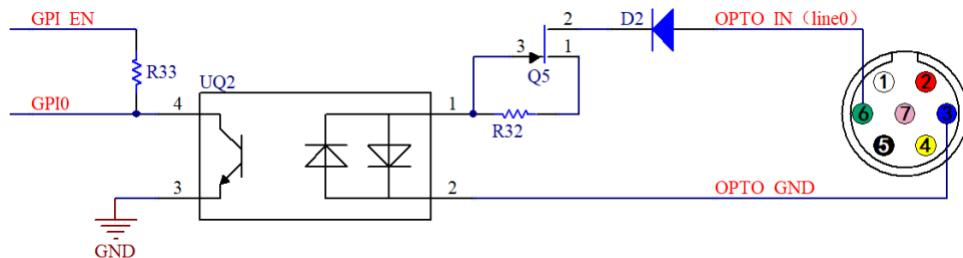
Figure 39 Opto-isolated input circuit
