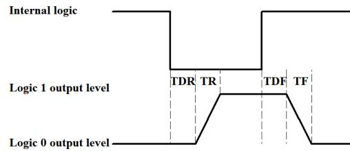
Figure 42 Output logic levels
