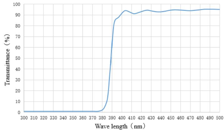
Figure 13 Long wave pass filter LPF390H transmittance curve
