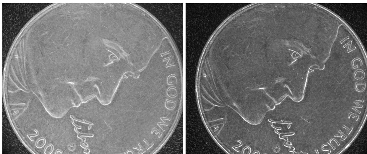
Figure 5- 55 Ordinary camera (left) compared with polarizing camera (right) metal surface effect
