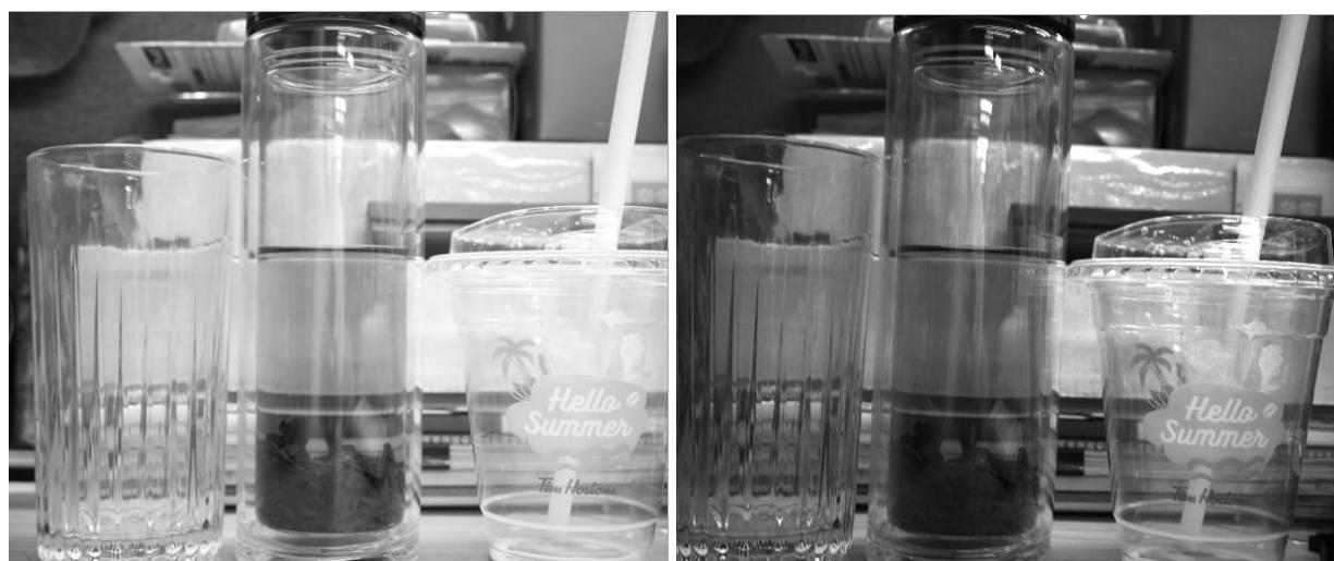
Figure 5- 53 Comparison of plastic surface effects between ordinary camera (left) and polarizing camera (right)
