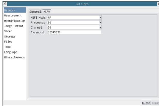
Plug the **USB WLAN** adapter into the camera's USB2.0 port;
