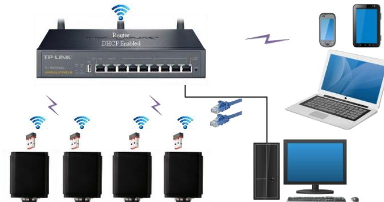
Figure 10 Multi XFCAMTOP4K8MPA Cameras Connecting to the Router through the WLAN Style
