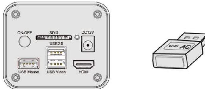
Install **ToupView/ToupLite** on your PC or install **ToupView App** on the mobile device, Connect the PC or mobile device to the camera's **WLAN AP** point; The network name (SSID) and the **WLAN** password (The default one is 12345678) can be found on the camera's **Setting>Network>WLAN** page in **AP** mode.
