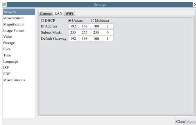
Figure 11 Configure the X7CAM4K Series Camera IP
