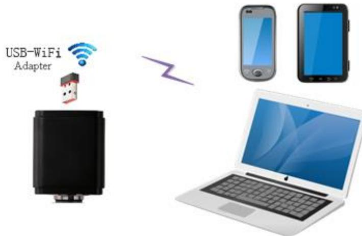
Figure 8 The PC or Mobile Device Connect to the Camera through WiFi
