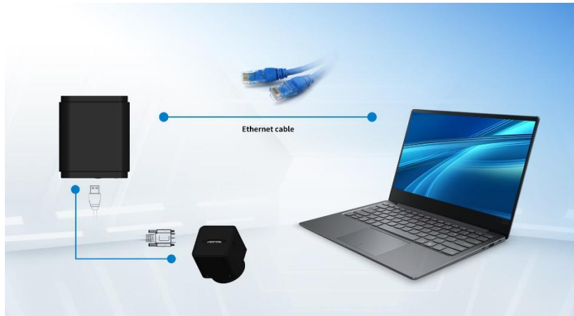
Figure 10 Connecting theX5CAM4K_MR Series Camera with Ethernet Cable to the PC
