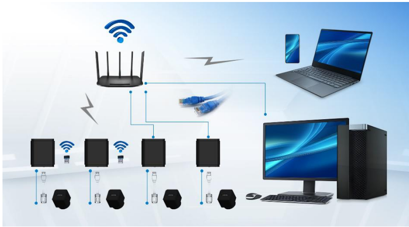
Figure 13 Multi X5CAM4K_MR Series Cameras Connecting to the Router through the LAN Port/ WiFi Style
