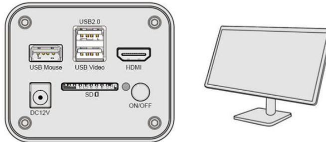
Insert the supplied USB mouse to the camera's USB port;
