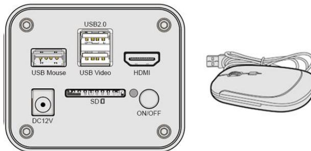
Insert the supplied SD card/USB flash drive (USB2.0 slot) into the SCAM4K series camera SD card slot/USB2.0 slot;
