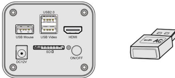
Install [ToupView/ToupLite](#) on your PC or install [ToupView App](#) on the mobile device, Connect the PC or mobile device to the camera's [WiFi AP](#) point; The network name (SSID) and the [WiFi](#) password (The default one is 12345678) can be found on the camera's [Setting>Network>WiFi](#) page in [AP](#) mode.
