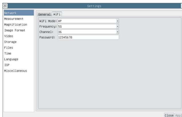
Plug the [USB WiFi](#) adapter into the camera's USB2 .0 port;
