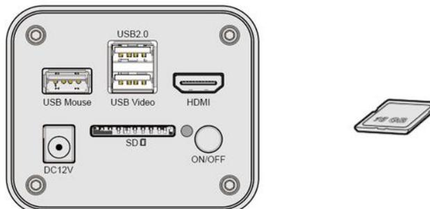
Connect the camera to the power adapter and turn it on;
