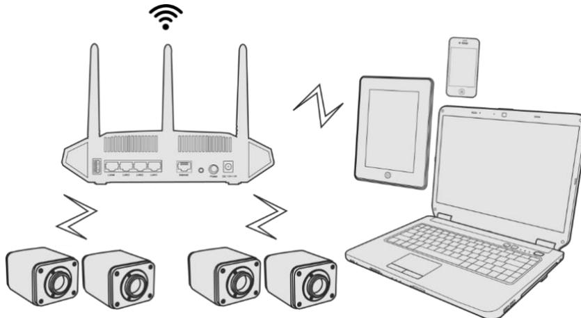
Make sure that your PC or your mobile device is connected to the WiFi of the router; Start [ToupView/ToupLite](#) software or [ToupView App](#) and check the configuration. Normally, active SCAM4K series cameras are automatically recognized. The live image of each camera is displayed. For the display, [Camera List](#) control panel window is used in [ToupView/ToupLite](#) software, and [Camera Thumbnail](#) is used in [ToupView App](#); Select the SCAM4K series camera
