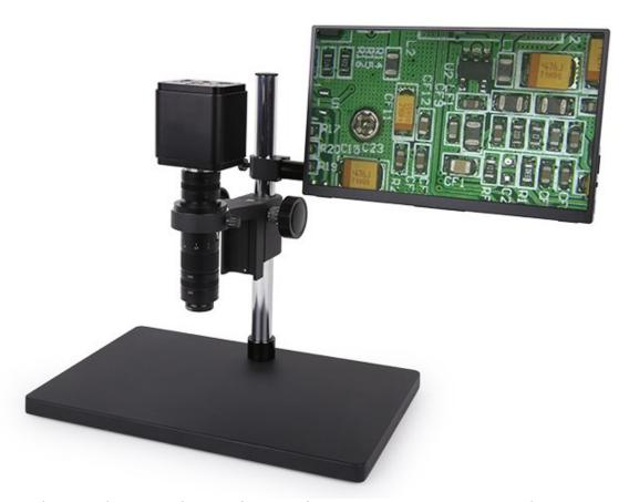
TPS300A Stand, Monocular Zoom Objective (TZM0480), XCAM Series HDMI Camera and TPHD4K133B Displayer
