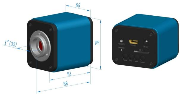
Dimension of XCAM720PHA Series Camera
