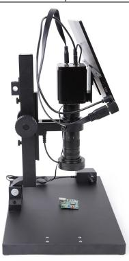
TPS-210A50(Stand)+TZM0480 (0.4x-8.0x Monocular Zoom Objective) +TXCAMLITE4K Camera(HDMI/USB Output CMOS Camera with Touch Function)+Touch Screen, the Touch Screen Is Fixed on the Fixing Block at the Front of the Camera through the Mounting Hole on the Built-in Bracket (Left side View, Short HDMI Cable and USB Type A to Type C Data Cable Can Be Used to Connect the Camera and Touch Screen)
