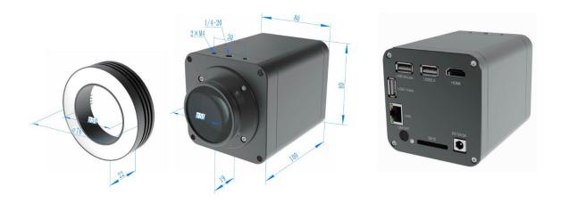
Figure 4-9 Dimension of AFDM411
