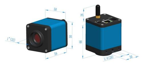
Dimension of WECAM Series Camera
