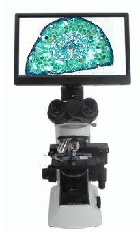
Front View of Olympus Microscope+XCAMSeries Camera and TPHD1080PA/B
