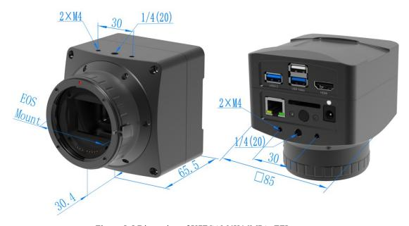
Figure 5-5 Dimension of X7FCAM4K16MPA\_EFL camera
