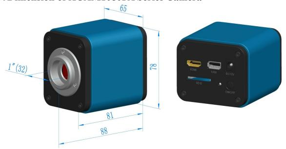
Dimension of XCAM1080PHA Series Camera
