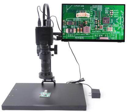
TPS-210A50-G(Stand)+TZM0480 (0.4x-8.0x Monocular Zoom Objective) +TXCAMLITE4K Camera(HDMI/USB Output CMOS Camera with Touch Function)+Touch Screen, the Touch Screen Is Fixed on the Cross Bar of Stand through the Mounting Hole on the Built-in Bracket (Front View, Short HDMI Cable and USB Type A to Type C Data Cable Can Be Used to Connect the Camera and Touch Screen)
